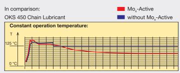
Constant operation temperature drops rapidly from + 120 °C to + 80 °C. Life time of the lubricant and thus relubrication intervals are prolonged multiple.
