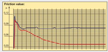
Friction value falls quickly from 0.09 to 0.03.
